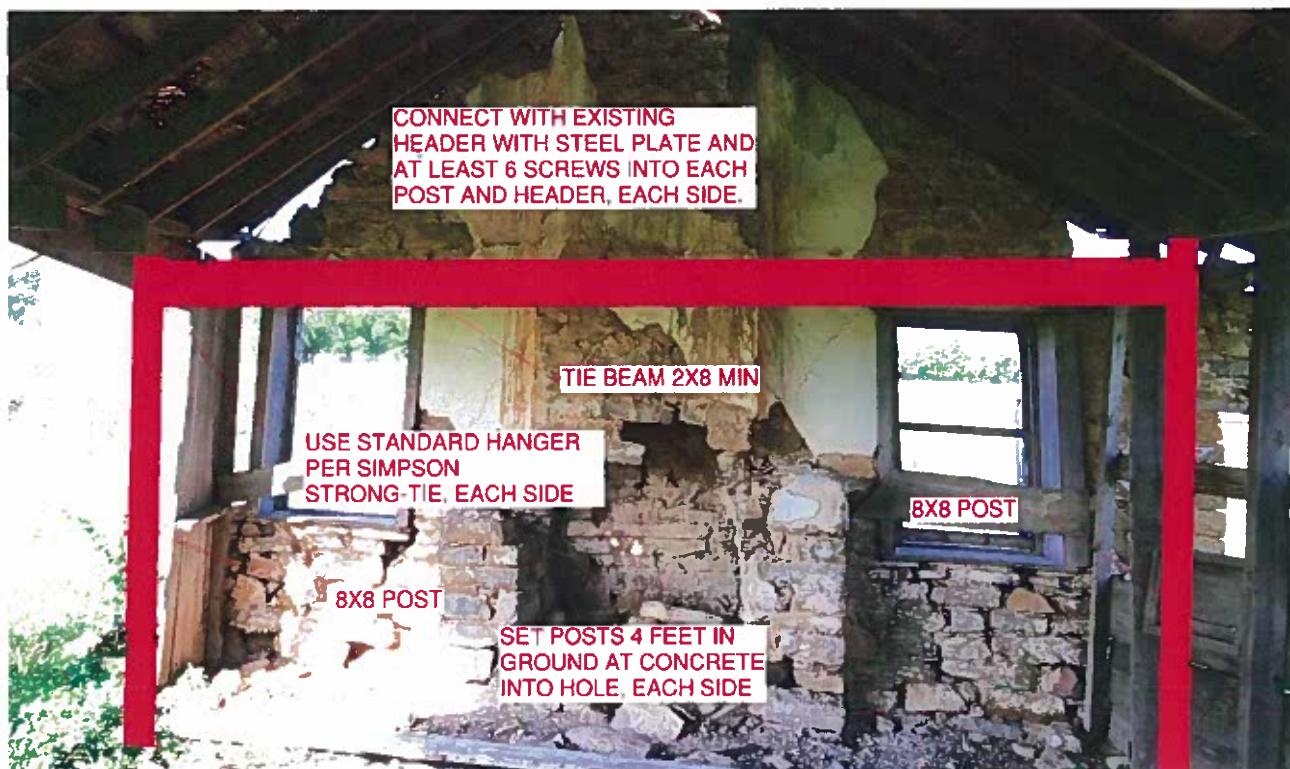
Figure 2: Posts and tie beam modifications
