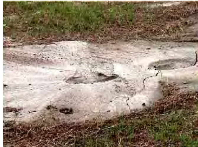
Figure 23: Sand Boil Example Due To High Seepage Rate
