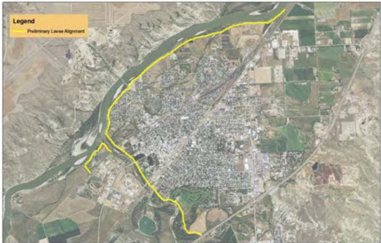
Figure 21: Preliminary Levee Alignment
