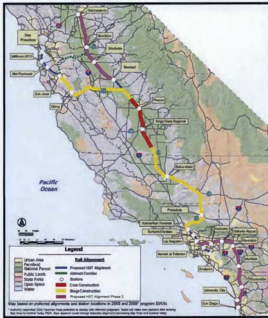
Figure 3: Future Efficient Expansions of HST System
