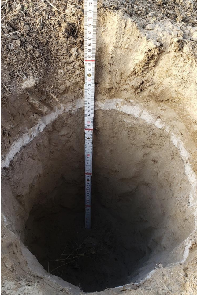
Figure 7. Profile of STP GT1 profile. Notice relatively fine-grained eolian sediments (loess) over more gravelly outwash/outburst flood sediments with cobbles at base. Unidentified light gray tephra between approximately 13 and 16 cmbs.
