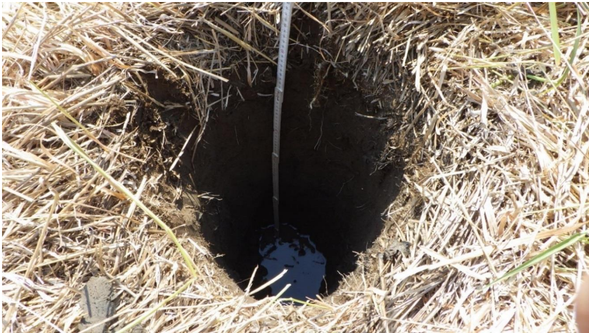
Figure 6. Profile of STP F5, water table at approximately 85 cmbs, and an increase in roots at 37 cmbs.
