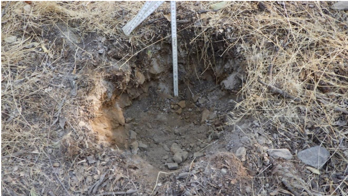
Figure 9. STP E2 depicting shallow soils on a weathered bedrock bench.
