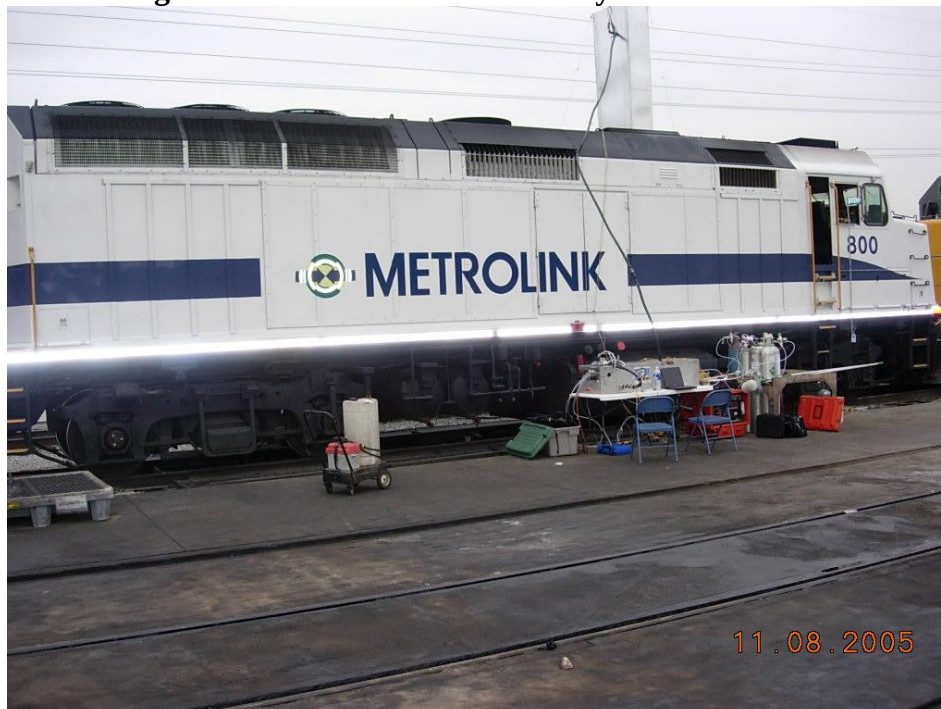
Figure 2: Emission measurement system installation on Metrolink No. 800
