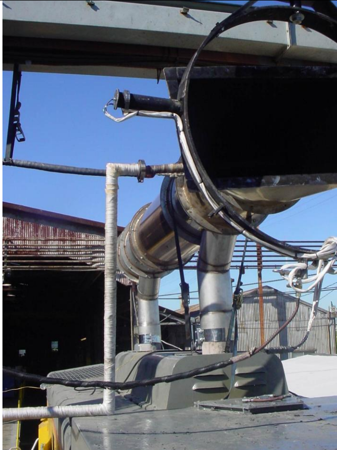
Figure 4. Exhaust Manifold Collection System For Emissions Sampling on UPY1378
