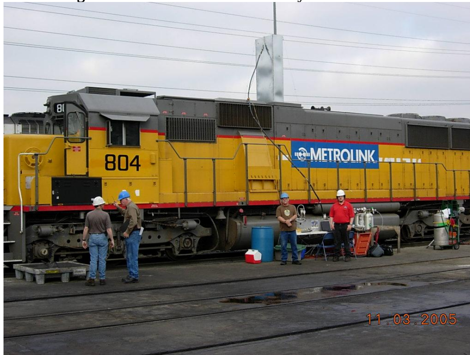
Figure 1: Emission measurement system installation on Metrolink No. 804
