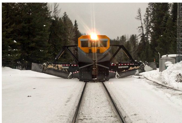
Jordan Spreaders, such as the one pictured here, are the most powerful plows in our fleet and are capable of pushing heavy snow and other debris well away from the track
