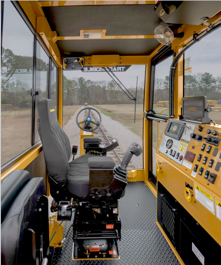
Atlas control panel and operational controls.
