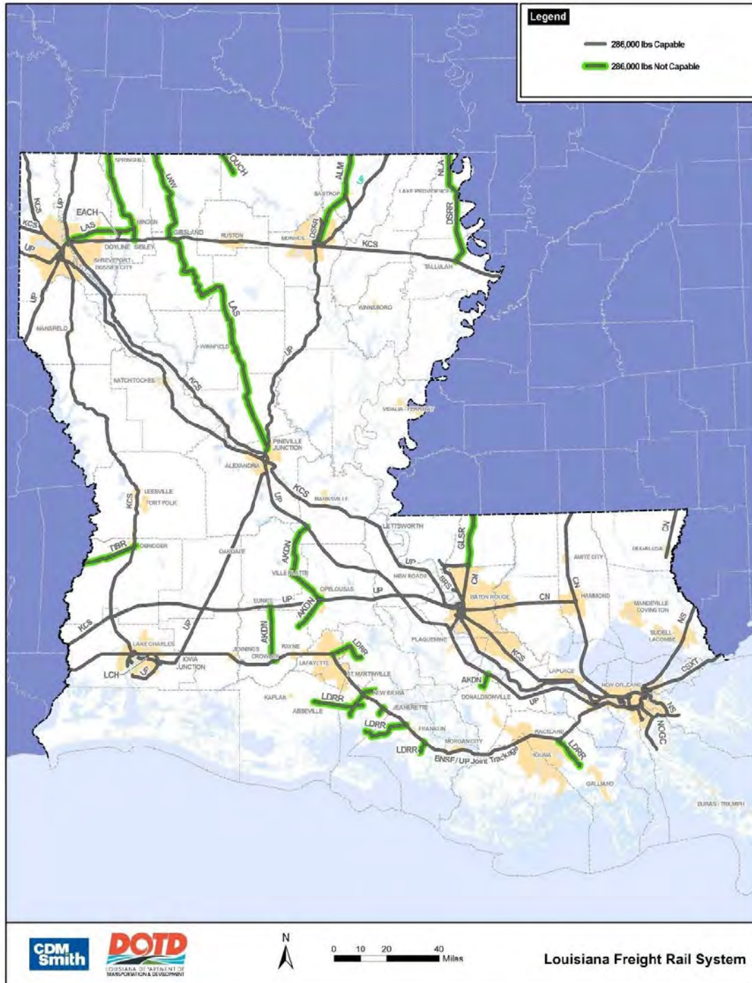
Figure A-12: DSR Track Weight Restriction within Louisiana
