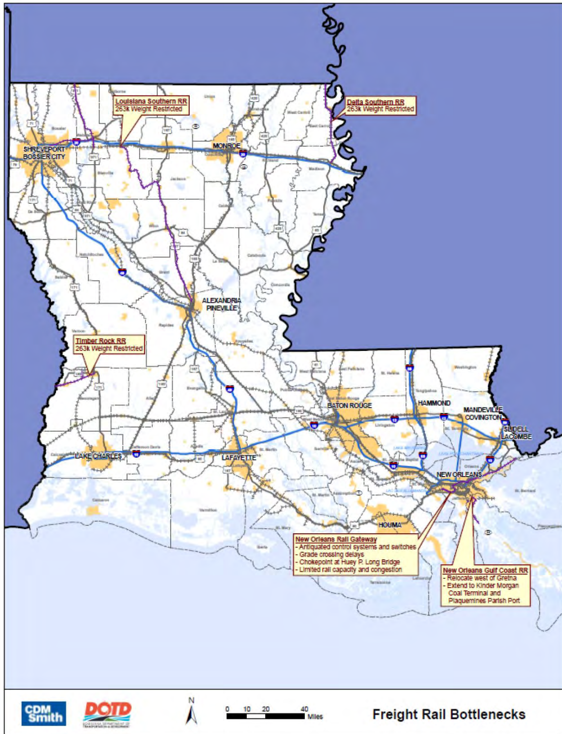
Figure A-13: DSR Freight Rail Bottlenecks
